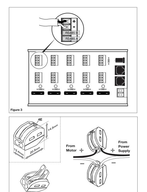
**3.** Connect wires to positive (+) and negative (-) at each motor port using a small screwdriver to firmly tighten.
