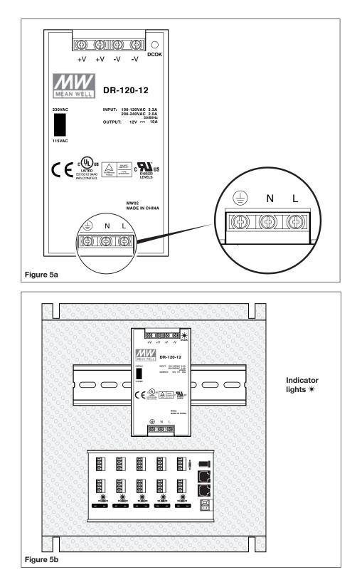
**6.** Have electrician install 120vac power to the transformer.
