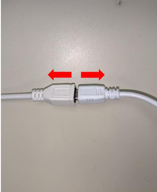
2. Disconnect the motor harness from the endcap.
