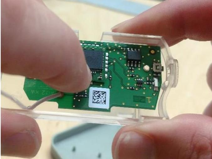
8. Insert the new push button into the housing by pressing into the housing as shown.
