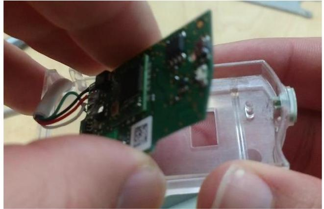
6. Remove the old push button by pushing out of the housing as shown below.
