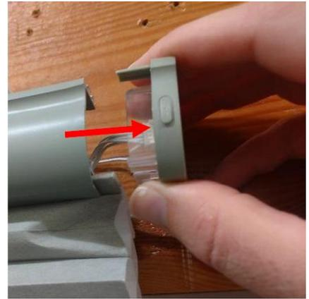
4. Disengage the cover from the housing. Position thumb on the cover as shown and apply force in an outward and downward motion.
