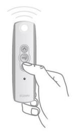
**3.** Once the shade stops, press and hold UP and DOWN simultaneously until the shade jogs.
