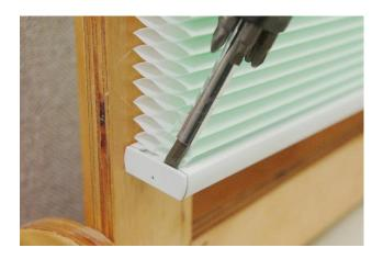
7. Slide aluminum slat from bottomrail. Placing a piece of tape on the end of the aluminum slat makes it easier to slide.
