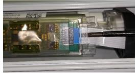
5. Once the ribbon cable is reinserted, the shade should function as normal. Reattach dust cover and test shade operation.
