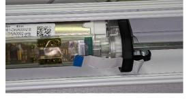
4. Using a small screw driver, reinsert ribbon cable into socket on motor. *Note: if the blue ribbon cover becomes detached, the cable can still be pushed back into place using your finger, this may be slightly more difficult to achieve.*
