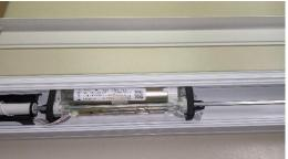
2. First, verify that the power cable and endcap ribbon cable are firmly inserted into their respective sockets.
