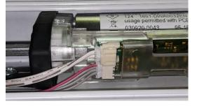
3. Motor ribbon cable may have come loose. Reconnecting this cable will allow the motor to function.
