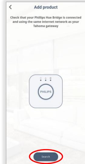
5. After the "Philips Hue bridge found!" message appears, SELECT the push-link button on the Hue Bridge, SELECT "Connect"
