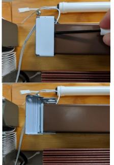
4. With endcap removed, slide the motor out of the headrail.
