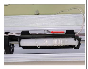
**12.** Reconnect endcap ribbon cable to motor.
