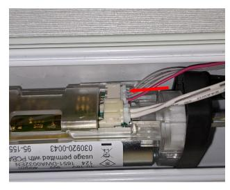
13. Install the endcap into the headrail.
