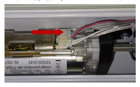
3. Remove the endcap from the headrail gripping the assembly and pulling away from the headrail. Note: It may be necessary to wiggle the endcap while pulling to disengage from the notch in the headrail. Once the endcap is removed, slide the ribbon cable out of headrail.
