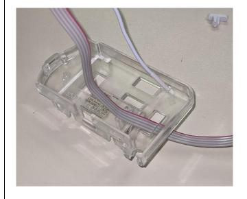
**8.** Replace the control board into the original position in the housing.
