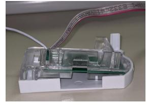
**5.** Gently raise control board out of housing to allow access to the push button.
